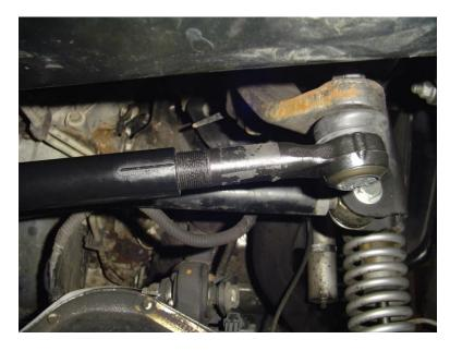
**Pitman Arm Ball Joint Connections**
